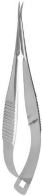
Vannas Scissors 13-077 Sharp pointed tips. Curved 7.5mm blades, 9.5mm from pivot to tip, 8 cm long
